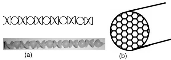
Fig. 2. Destructive devices used (the metal static mixer A has the same shape as the plastic static mixer B with a different length of each helical element) (a) 12 elements of mixer B; (b) honeycomb.
